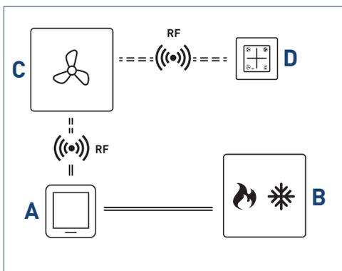
Thermostat connection schematic diagram.
