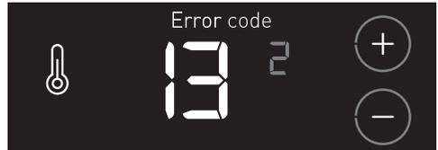
*For example: The error code **A1 13** consists of a device code (A1) and a serial number (13) that are shown alternately.*
