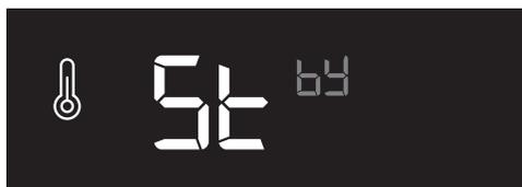
It is possible to turn off the thermostat's temperature demand (**HEATING** or **COOLING**) indefinitely, for example during your holiday. To do this, the thermostat must be set to **STANDBY** mode.
