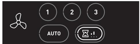
*The timer can be interrupted at any time by pressing the low setting, medium setting, high setting or auto-ventilation button.*
