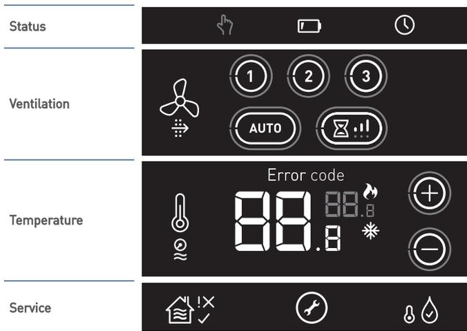
The screen is a capacitive touch screen. This means that the thermostat is controlled by the physical touching of the symbols on the screen.
