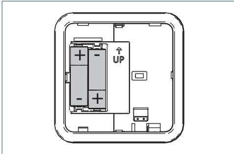
*Note the plus and minus poles in the battery holder to fit the batteries in the correct position.*
