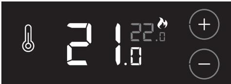
*The heating temperature is adjustable between 18°C and 24°C.*
